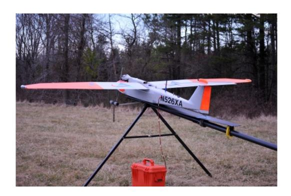
The first Mid-Atlantic Aviation Partnership at Virginia Tech test flight using a fixed-wing unmanned aircraft to inspect an energy pipeline route—with a piloted chase plane following behind to ensure safety beyond the ground observers' sight line —was completed last week. The flight was a step toward making aerial inspections of energy pipelines safer and more economical, researchers say.
