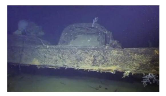
There were holes in the bow area, apparently made by U.S. torpedoes, and the ship's stern is upside down. A propeller is torn off from a shaft and gun turrets and catapults are broken off.
