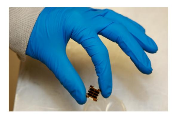
MIT physics graduate student Patrick Brown holds a lead sulfide quantum-dot solar cell in the Organic and Nanostructured Electronics (ONE) Lab at MIT, where he works under Vladimir Bulović, the Fariborz Maseeh Chair in Emerging Technology at MIT School of Engineering. Credit: Denis Paiste/Materials Processing Center
