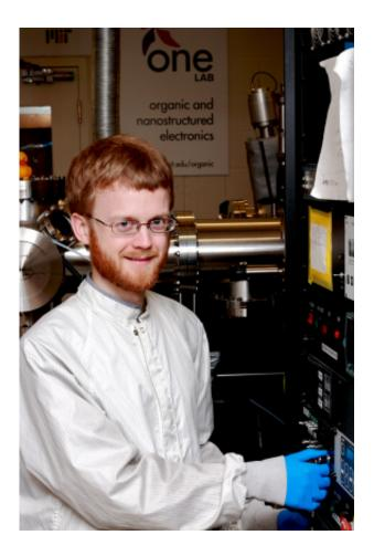
MIT physics graduate student Patrick Brown stands at the controls for a magnetron sputterer deposition chamber, used in the fabrication of charge-transport layers for quantum-dot solar cells. Credit: Denis Paiste/Materials Processing Center
