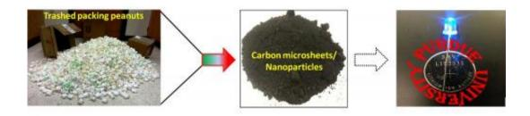
This schematic depicts a process for converting waste packing peanuts into highperformance carbon electrodes for rechargeable lithium-ion batteries that outperform conventional graphite electrodes, representing an environmentally friendly approach to reuse the waste. Credit: Purdue University image/Vinodkumar Etacheri
