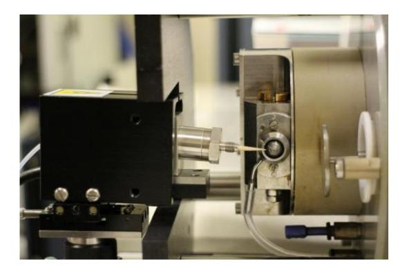
The desirable features of wooden tips permit direct mass spectrometric analysis of drugs in urine and oral fluid without having to go through sample pretreatment and chromatographic separation, enabling the analysis of one sample to be completed within a few minutes. Credit: Hong Kong PolyU
