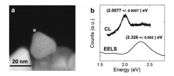
On the left, a STEM image of a triangular gold nanoparticle sitting on titanium oxide surface. The white circle at the top corner of the gold nanoparticle indicates where the electron beam is making spectroscopic measurements. On the right are the corresponding spectra representing electron absorption and emission. Credit: Sharma/NIST
