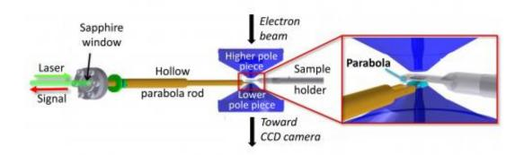
Schematic view of the integrated optical spectroscopy system developed at NIST. The laser goes through the sapphire window, bounces off the parabolic mirror and onto the sample above. The parabolic mirror also collects a portion of the vibrational spectra/photons emitted by the sample for analysis. Credit: Sharma/NIST
