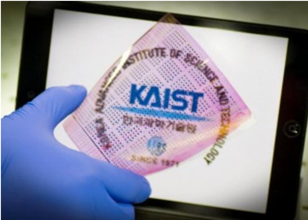
Transistor array fabricated on a large scale, highly flexible substrate with pV3D3 polymeric films. Credit: KAIST
