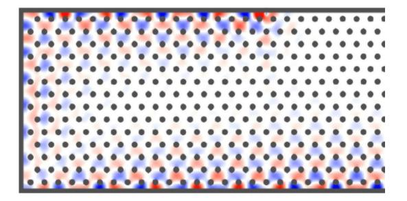
Around the bend. An acoustic topological insulator would guide sound waves around its edges, as shown in this simulation. Credit: Z. Yang et al., *Phys. Rev. Lett.* (2015)
