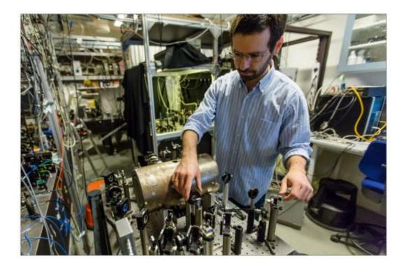
Georgios Vasilakis, a postdoc in Quantop is working on the experiments in the quantum optics laboratory. Here, the researchers have a tiny glass tube that contains a cloud of billions of caesium atoms and using laser light, the tilts of all of the atoms are turned in the same direction and you can calculate the ultrasmall magnetic fields with great precision. Credit: Ola Jakup Joensen, NBI
