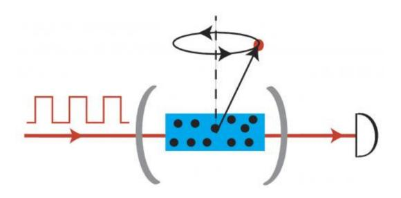
The newly developed sensor that can measure the ultra-small magnetic fields is comprised of a cloud of billions of cesium gas atoms in a tiny glass tube. Using laser light, the tilts of all of the atoms are turned in the same direction. Credit: Kasper Jensen, Niels Bohr Institute
