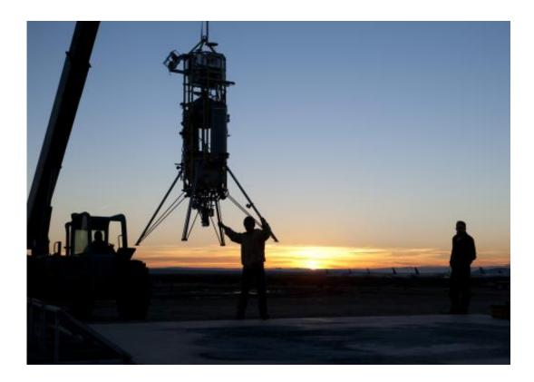
The ADAPT test system can help a spacecraft divert its course and make a smooth, pinpoint landing. The system is built on Masten's XA-0.1B "Xombie" vertical-launch, vertical-landing reusable rocket. Credit: NASA Photo / Tom Tschida
