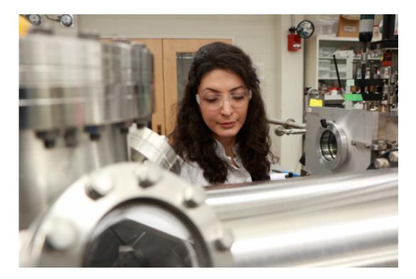
Farnaz Niroui works at a thermal evaporator, which she uses to deposit a gold coating on squeezable switches, or "squitches," which she designed, fabricated and tested. It is part of a vacuum-sealed transfer line for making nanoscale electronic devices. Credit: Denis Paiste/Materials Processing Center
