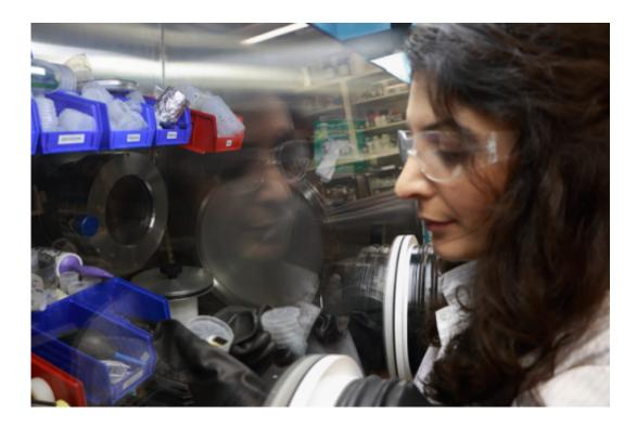
MIT electrical engineering graduate student Farnaz Niroui works in a glovebox, where she prepares a sample for deposition of gold. The glovebox is attached through a transfer line to a thermal evaporator that deposits the gold coating onto squeezable switches, or "squitches," which Niroui designs, fabricates, and tests in the Organic and Nanostructured Electronics Lab at MIT. Credit: Denis Paiste/Materials Processing Center
