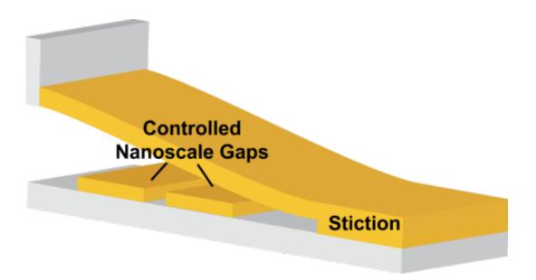
MIT electrical engineering graduate student Farnaz Niroui has designed a fabrication process for nanoscale electromechanical switches in which a cantilever can collapse and permanently adhere onto a support structure, leaving a controllable nanoscale gap between the cantilever and electrodes neighboring the point of adhesion, which is called stiction. Credit: Farnaz Niroui
