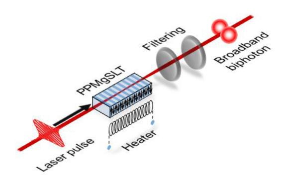
Researchers at the University of Electro-Communications have successfully generated broadband biphotons and examined their spectral properties. Their insights may help create controllable optical fields for use in quantum information and communication technologies.
