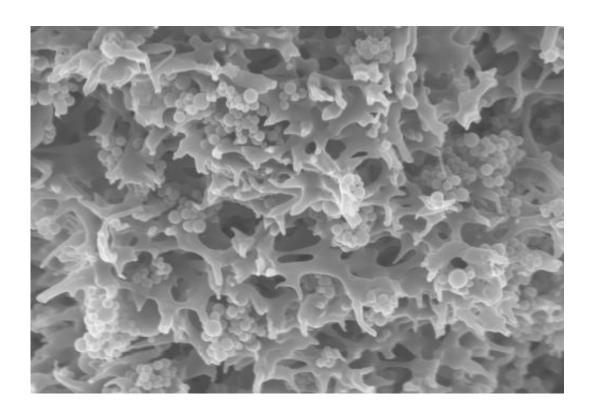
New types of membrane adsorbers remove unwanted particles from water and also, at the same time, dissolved substances such as the hormonally active bis-phenol A or toxic lead. To do this, researchers at the Fraunhofer Institute for Interfacial Engineering and Biotechnology IGB imbed selective adsorber particles in filtration membranes.
