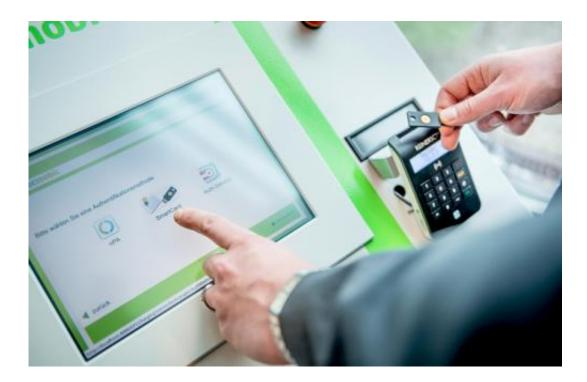
When a user identifies him- or herself at the RUB charging station, their personal data, together with additional billing information, are packed into a coded packet. Credit: RUBIN, photo: Gorczany
