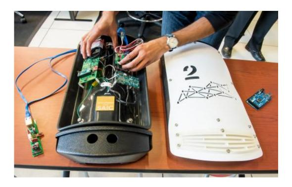
The circuit boards for the Argonne-developed Waggle platform are installed in a safe, weather-proof casing for a deployment in partnership with the City of Chicago, called the "Array of Things." Early test units such as pictured here are scheduled to be installed on the campuses of DePaul University, University of Chicago and the School of the Art Institute of Chicago. Photo by Mark Lopez/Argonne National Laboratory. Credit: Mark Lopez/Argonne National Laboratory
