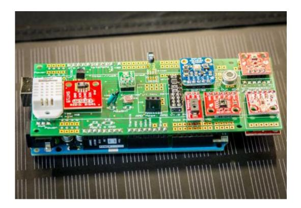
"No more one-offs" The newly developed Waggle platform is computing in a box. With 4 processors, a Linux-based operating system and the ability to mixand-match an array of sensors, the Waggle platform outfits researchers with a next-generation data collection experience in real time from their computer. Credit: Mark Lopez/Argonne National Laboratory.
