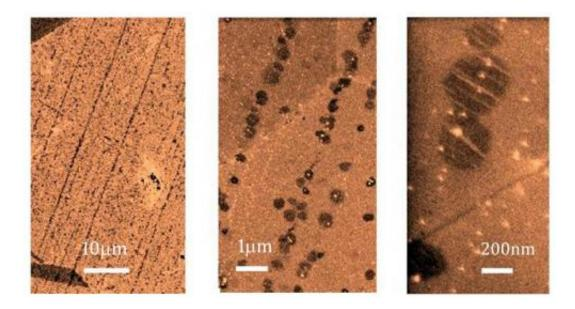
Early-stage growth of graphene on copper. The lines of hexagons are graphene nuclei, with increasing magnification from left to right, where the scale bars from left to right correspond to  $10 \mu m$ ,  $1 \mu m$ , and 200 nm, respectively. The hexagons grow together into a seamless sheet of graphene. Credit: D. Boyd and N. Yeh labs/Caltech
