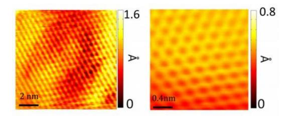
Atomically resolved scanning tunneling microscopic images of graphene grown on a copper (111) single crystal, with increasing magnification from left to right. Credit: D. Boyd and N. Yeh labs/Caltech
