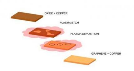
Schematic of the Caltech growth process for graphene. Credit: D. Boyd and N. Yeh labs/Caltech
