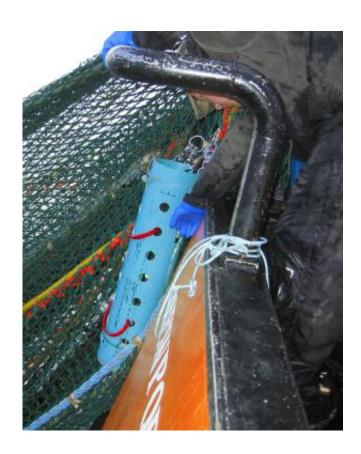
Researchers developed a sturdy, protective housing for oxygen sensors attached to trawl nets to protect them from damage. Survey vessels now carry such sensors on all of their tows to document associations between species and dissolved oxygen levels. Credit: NOAA Fisheries/Northwest Fisheries Science Center
