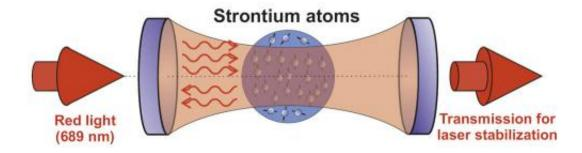
The laser light is sent through a 'resonator', which consists of two mirrors. This resonator selects specific wavelengths. A vacuum chamber containing ultra cold atoms is placed in between the two mirrors and acts as a frequency filter. As a result, the laser can be stabilized much better than with just the empty 'resonator'. Credit: Bjarke Takashi Røjle Christensen, NBI
