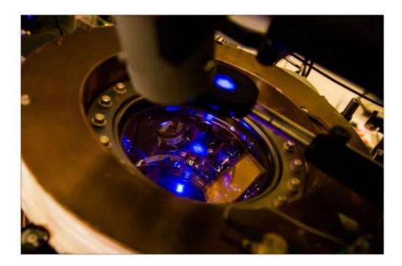
Atoms are cooled down to temperatures near the absolute zero by using laser light (blue light) and magnetic fields.
