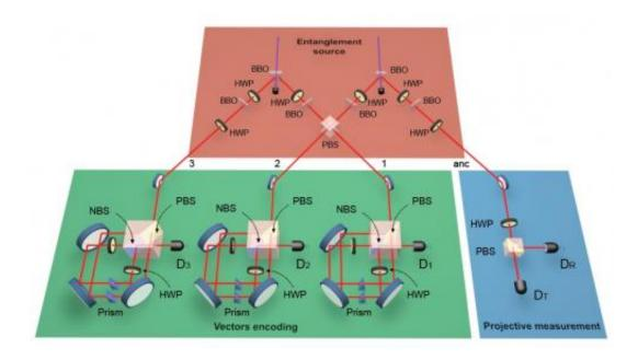
Experimental setup for quantum machine learning with photonic qubits. Credit: X.-D. Cai, et al. ©2015 American Physical Society
