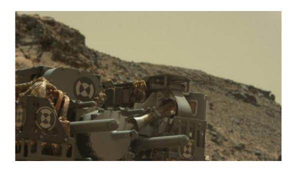
This raw-color view from Curiosity's Mastcam shows the rover's drill just after finishing a drilling operation at "Telegraph Peak" on Feb. 24, 2015. Credit: NASA/JPL-Caltech/MSSS
