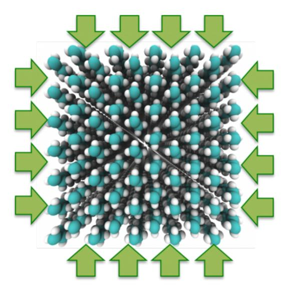
The new AIREBO-M Potentials validated against a pressure-volume isotherm at T=533K for polyethylene crystals. Note the AIREBO-M potentials show nearly perfect agreement with REAXFF calculations and experimental data. However the AIREBO-M potentials are much more computationally efficient than REAXFF calculations, and will allow upscaling of calculations to perform much
