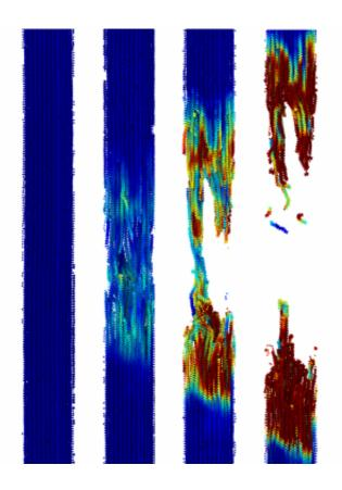
The new AIREBO-Morse potentials (AIREBO-M) are used in a simulation to deform and break polyethylene fibrils. Large scale simulations like these will allow us to explore effects of defects and other important variables on the
