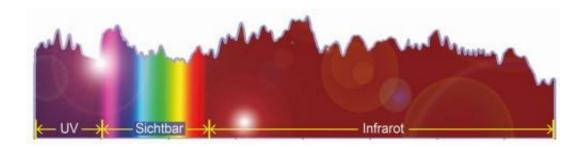
Similar brightness from ultraviolet to infrared: The intensity of the broad bandwidth light that can be generated with a photonic crystal fibre remains more or less the same level across the entire wavelength range – a very advantageous property for many applications. Credit: Xin Jiang
