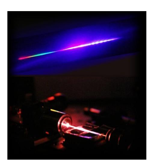
Light with a UV component: The Erlangen-based researchers disperse the light generated in the photonic crystal fibre with a prism, similar to the way in which
