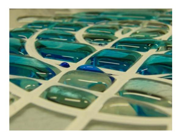
Water (dyed blue) was framed in the drawing of superhydrophobic materials, forming a 3D superhydrophobic painting. Credit: Yao Lu - UCL
