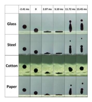
Time-lapse photographs of water droplets bouncing on the treated glass, steel, cotton wool and filter paper surfaces (droplet size: ca  $6.3 \pm 0.2 \,\mu\text{L}$ ). Credit: Lu Yao, UCL
