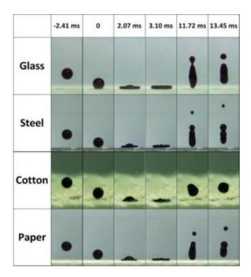
Time-lapse photographs of water droplets bouncing on the treated glass, steel, cotton wool and filter paper surfaces (droplet size: ca  $6.3 \pm 0.2 \mu$ L). Credit: Lu Yao, UCL
