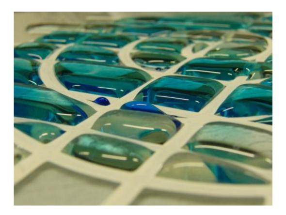
Water (dyed blue) was framed in the drawing of superhydrophobic materials, forming a 3D superhydrophobic painting. Credit: Yao Lu - UCL
