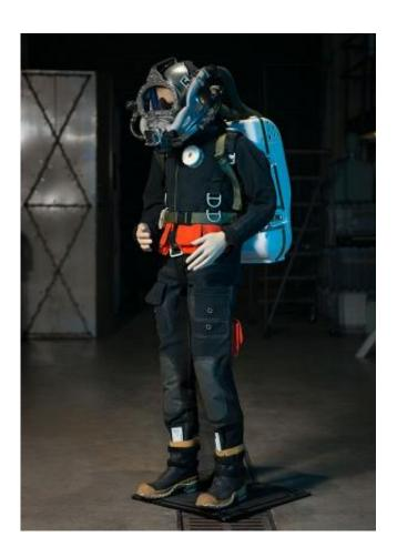
A prototype for a new life support system for divers is displayed on a mannequin at the Naval Surface Warfare Center in Panama City, Fla. The semi-closed system has been developed to accelerate Navy diver deployment, increase safety, and conserve the mixed gas atmosphere. Credit: U.S. Navy photo by Anthony Powers
