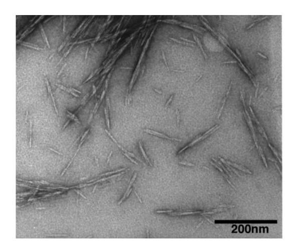
This transmission electron microscope image shows cellulose nanocrystals, tiny structures derived from renewable sources that might be used to create a new class of biomaterials with many potential applications. The structures have been shown to increase the strength of concrete. Credit: Purdue Life Sciences Microscopy Center
