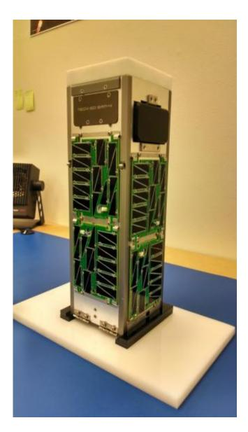
The TechEdSat series, a technology education collaboration with San Jose State University and the University of Idaho, uses the standard CubeSat structure, which measures one unit (1U) as approximately four inches cubed (10 centimeters cubed). TechEdSat-4 is a 3U satellite. Credit: NASA Ames
