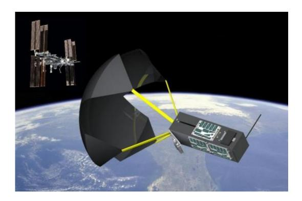
This is a graphic rendering of TechEdSat-4 with exo-brake deployed. Exo-brake is an aerodynamic specially-designed parachute-like device, that causes the satellite to de-orbit and re-enter Earth's atmosphere. Credit: NASA Ames
