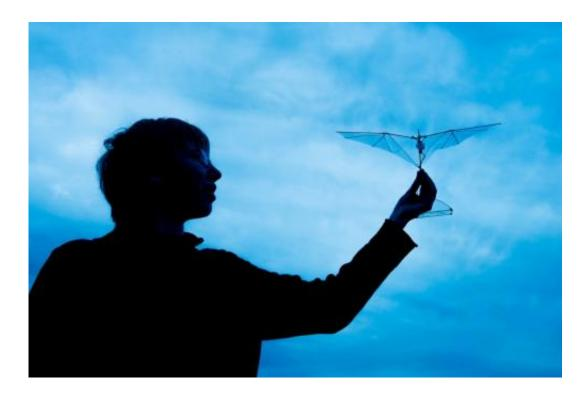
Graduate student Amanda Stowers of The Lentink Lab at Stanford University demonstrates her passive morning wing design for a flapping robot. The wrist hinge enables the robot to comply with hard impact of a steel rod, while the flapping motion forces the wings to fully extend again after impact. Credit: Linda Cicero, Stanford University
