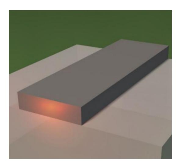
The strong confinement in the silicon photonic nanowire waveguide enhances the light matter interaction. The strong interactions allow to extend a frequency comb towards the mid-infrared. Credit: Ghent University
