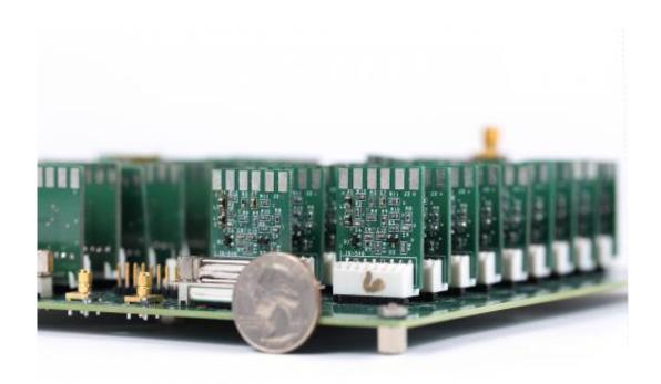
A new technology that could represent an advanced medical diagnostic tool for the early detection of cancer and other diseases is made possible with this electronic device developed at Purdue's Jonathan Amy Facility for Chemical Instrumentation in the Department of Chemistry. The device is called a 32-channel tuned amplifier array, or TAMP array. Two patents have been issued for the new technology. Credit: Purdue University
