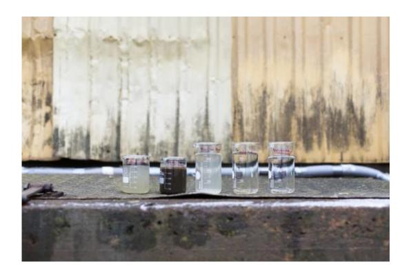
Purified wastewater using membrane filtration. Credit: Teemu Leinonen, LUT
