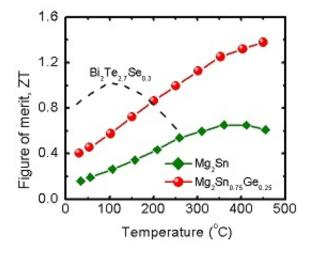
Temperature-dependent thermal properties and ZT values. ZT values of Bi2Te2.7Se0.3 are plotted for comparison. Credit: University of Houston
