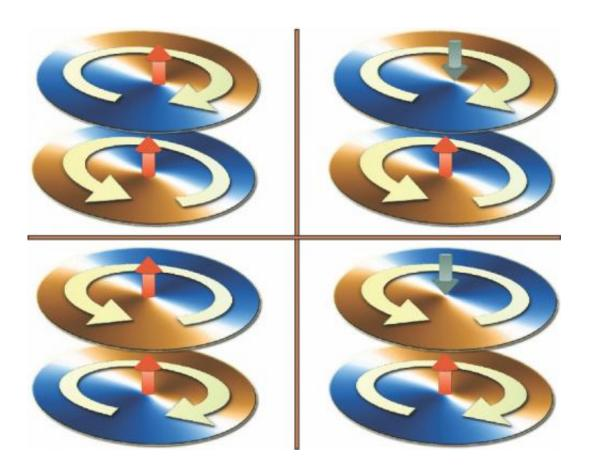
Shown are four examples of the double-vortex states investigated with opposite vorticity. In each disk, the flat yellow arrows represent the sense of the circulation of the in-plane magnetization component. The red and green arrows indicate the polarity of the vortex core. The tiny core, with a diameter of only a few nanometers, is surprisingly important for the magnetization dynamics when a current flows through the double-vortex pillars. Credit: HZDR/FZJ
