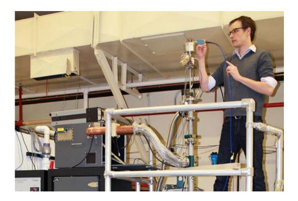
Los Alamos National Laboratory scientist Brad Ramshaw conducts an experiment at the Pulsed Field Facility of the National High Magnetic Field Lab, exposing high-temperature superconductors to very high magnetic fields, changing the temperature at which the materials become perfectly conducting and revealing unique properties of these substances. Credit: Los Alamos National Laboratory
