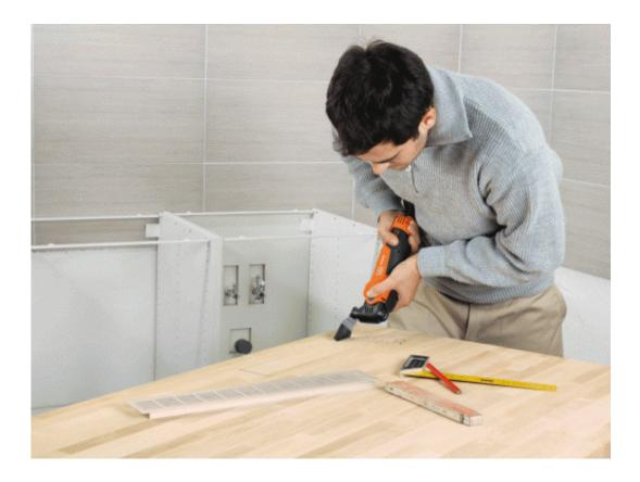
FEIN's versatile power tool vibrates up to 70 percent less and is only half as loud as its predecessor. Credit: C. & E. Fein GmbH
