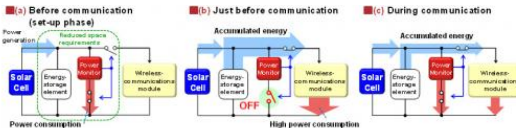
Figure 1: How the power-control operation works
