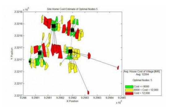
In a different village in India, the team's software was used to figure out where solar panels could be installed to create an electric microgrid, and what the most efficient arrangement of transmission wires would be to connect the houses.
