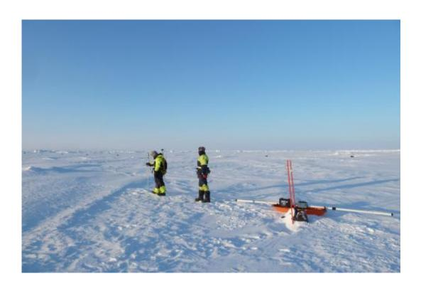
Field scientists from the N-ICE2015 campaign measure snow and ice thickness along a survey line in preparation for Operation IceBridge's overflight. Credit: Norwegian Polar Institute/ Gunnar Spreen
