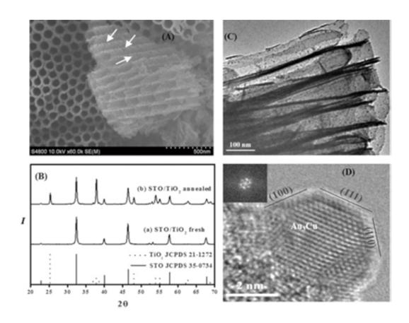
A combination of semiconductor catalysts, optimum catalyst shape, gold-copper co-catalyst alloy nanoparticles and hydrous hydrazine reducing agent enables an increase of hydrocarbon generation from CO<sub>2</sub> by a factor of ten.
