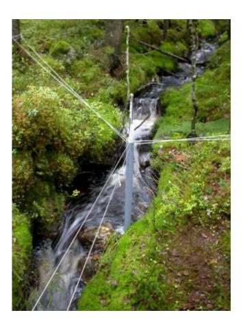
A riparian zone along a headwater stream in the Krycklan catchment area with instruments measuring water levels (logger in the PVC tube), simulated plant damage (wooded sticks), and simulated sedimentation (PVC carpets). Credit: Lenka Kuglerová
