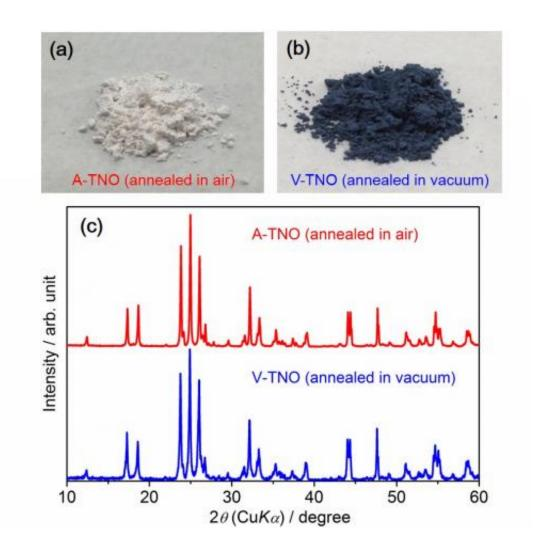
Photos of TNO annealed in air (A-TNO) (a) and vacuum (V-TNO) (b). X-ray diffraction patterns for both samples is also shown in (c). Credit: (c) Toyohashi University of Technology
