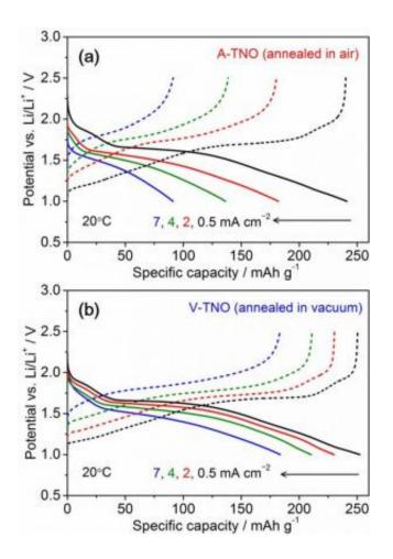
Charge (solid lines) and discharge (dashed lines) curves at different fixed current densities of 0.5, 2, 4 and 7 mA cm-2 for (a) A-TNO and (b) V-TNO electrodes are shown. Credit: (c) Toyohashi University of Technology
