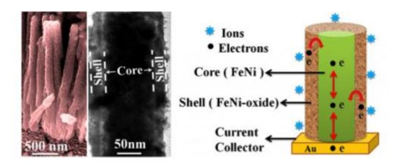
High performance supercapacitor electrodes.Left: field emission scanning electron microscope and transmission electron microscope micrographs; Right: sectional view of single hybrid nanostructure. Credit: Ashutosh K. Singh and Kalyan Mandal/S.N. Bose National Centre for Basic Sciences, India
