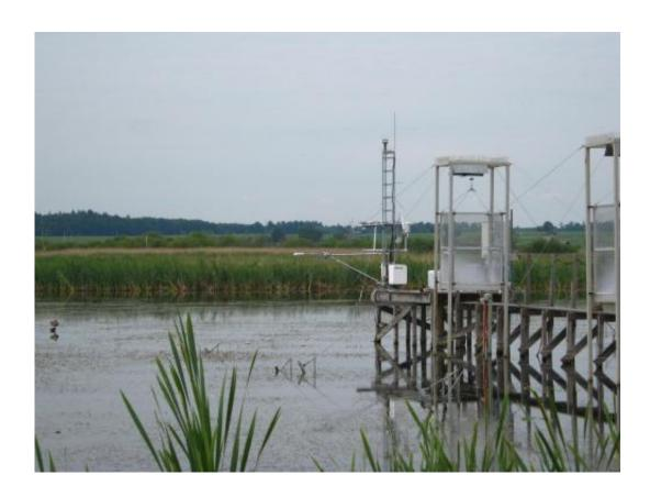
Automatic flux measurement chambers and an eddy covariance system to determine turbulent exchange fluxes of heat, water vapor, CO2, and CH4 between a re-wetted peatland and the atmosphere at Zarnekow, NE Germany. Credit: Daniela Franz, GFZ
