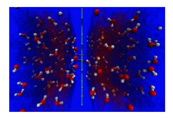
Proton transfer channel across a quad-defect in graphene, as obtained from a ReaxFF molecular dynamics simulation. Credit: Murali Raju, Penn State
