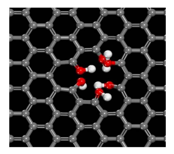
Hydroxylated defect site that allows for facile proton transfer through the pristine single-layer graphene substrate. Credit: University of Minnesota
