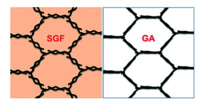
How can the electrodes of batteries be made more efficient? In the journal *Angewandte Chemie*, American scientists describe a powerful approach that uses solvated graphene frameworks as the anode material. Assembled in a lithium coin cell, the as-made electrode excelled with capacities surpassing the values of typically used graphite.
