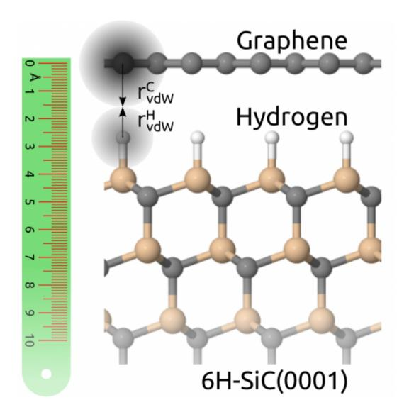
Graphene on a silicon carbide substrate whose surface has been treated with hydrogen in order to electrically decouple the graphene. The distance between the two layers, minus the respective van der Waals radii, gives an approximate value for the interaction strength. Credit: Sforzini et al., *Physical Review*
