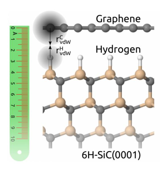
Graphene on a silicon carbide substrate whose surface has been treated with hydrogen in order to electrically decouple the graphene. The distance between the two layers, minus the respective van der Waals radii, gives an approximate value for the interaction strength. Credit: Sforzini et al., *Physical Review*
