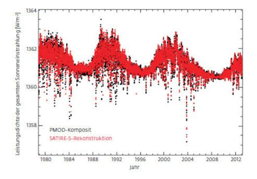
The Sun's total radiative flux fluctuates over an 11-year cycle. The SATIRE-S model (red dots) reproduces over 92 percent of measured irradiance variations (black dots). When the short, deep drops in TSI occur, dark spots wander across the Sun's visible surface. Credit: Solar System Research
