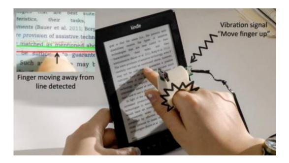
Researchers at the MIT Media Lab have created a finger-worn device with a built-in camera that can convert text to speech for the visually impaired.
