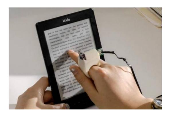
Researchers at the MIT Media Lab have created a finger-worn device with a built-in camera that can convert text to speech for the visually impaired.
