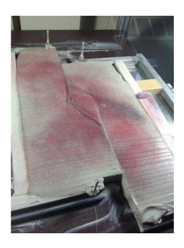
The UMass Amherst lab is one of only a handful worldwide to use a state-of-theart modeling technique based on kaolin clay rather than sand to understand the behavior of the Earth's crust. Credit: UMass Amherst
