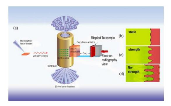
In this experimental setup at the Omega Laser Facility, the hohlraum drives the reservoir-gap configuration, creating a ramped plasma drive that compresses and accelerates the sample without shock melting. The team measured the Rayleigh-Taylor instability ripple growth amount to infer the dynamic flow stress of the sample.
