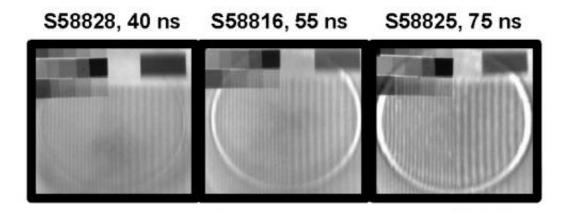
These figures show face-on radiography of Rayleigh-Taylor induced ripple growth at different delay times. Higher contrast ripples mean that the ripples are grown more rapidly.
