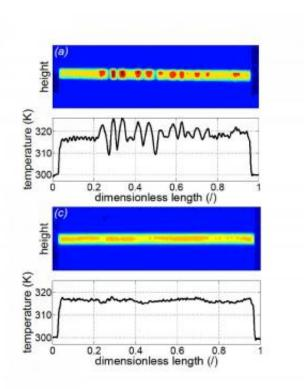
Static presentation of the temperature distribution over Ni-Ti wires measured with an infrared camera during loading in the case of virgin (upper) and fully stabilized (lower) wire. Credit: J. Tušek, K. Engelbrecht, L.P. Mikkelsen, N. Pryds
